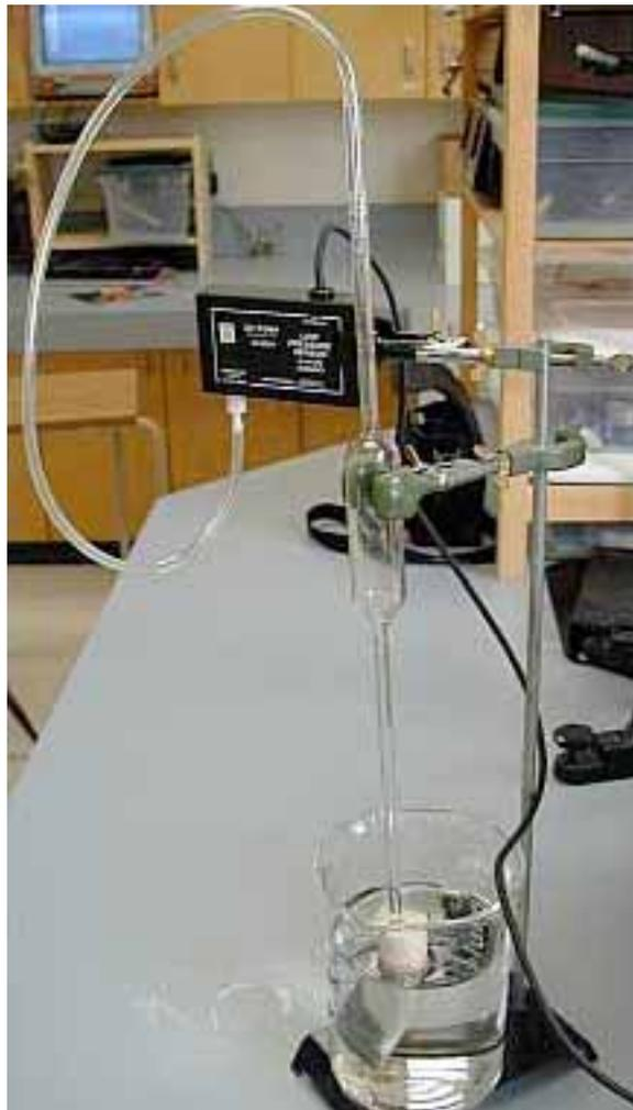
6. Begin collecting data soon after the baggie is suspended in the distilled water. Allow data to collect for several minutes. While collecting data, make the preparations for the switch to a new beaker solution for step 7.
